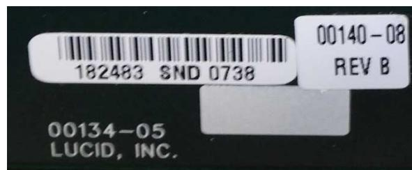
*Version identification markings on the circuit boards of the Optical Mark Recognition scanner unit*
