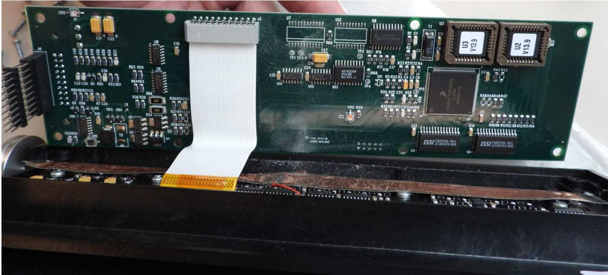
*Inner view of the scanner unit, showing white powder on circuit board and support frame
